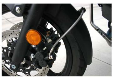
h. Line C routed over the fender to the left caliper
