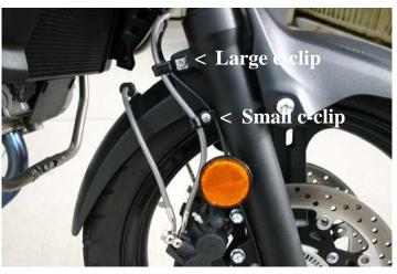
f. Line B & C at right caliper, notice c-clips at fork
