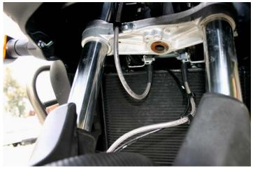
e. Line A routing from MC, and Line B routing towards the "right" caliper
