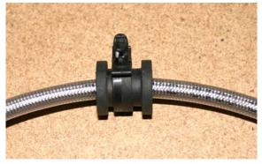
i. OEM line holder pre-installed to Line  $\boldsymbol{C}$
