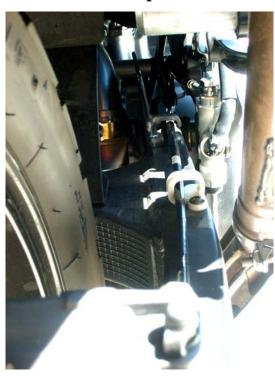
c. Rear routing, using OEM routing clip
