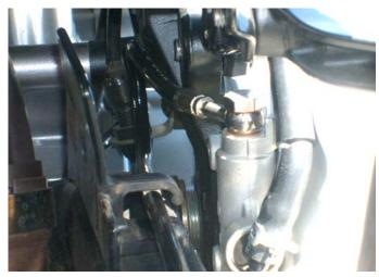
b. Routing behind rear master cylinder, under routing tab
